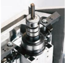
Electrospindles with HSK D-50 coupling.
