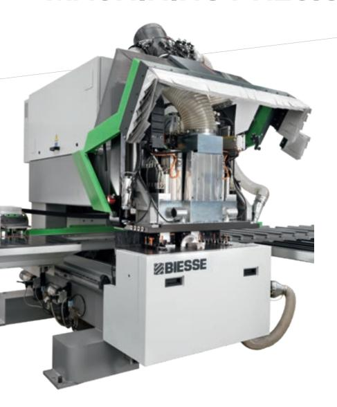
The machining of the machine base on single-positioning processing centres guarantees optimum precision for mechanical operations. The fixed operating sections (and mobile panels) ensure long-term machining accuracy and reliability.
